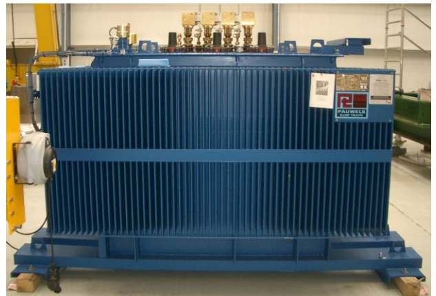
Fig. 17- ECO 122 main transformer.
